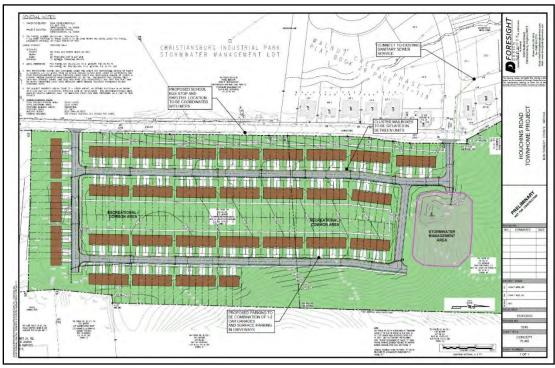
Figure 2: Preliminary Site Plan (Prepared by Gress Engineering for informational purposes only)
